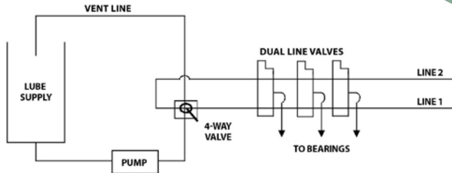
This type is usually used where long runs or low temperatures are encountered. Points can easily be added.
